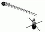
Modifications, such as add-ons and conversions not intended by the manufacturer, may only be performed with the written consent of the markilux® manufacturer. Additional loading of the awning due to suspended objects or due to tensioned ropes/cables can lead to damage or to the collapse of the awning and are therefore not permitted.
