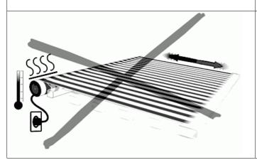
**4.2** Extending and retracting the awning several times in quick succession causes the automatic shutdown of the motor, which is thereby protected from overheating.
