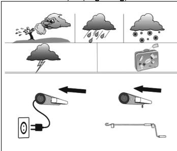
The awning may not be extended during snowfall or the danger of frost. The danger exists that the awning could be damaged or collapse.
