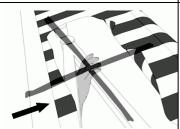
Depending on the type of awning, there exist crush and shear zones, e.g. between drop rod and cassette and between moving parts. Items of clothing or limbs can be grabbed by the unit and pulled in!
