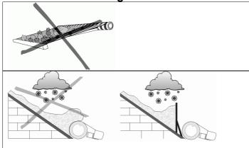
Leaves and other foreign matter lying on the awning cover, in the awning box and in the track profiles are to be removed immediately. The danger exists that the awning could be damaged or collapse.
